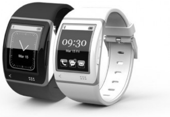
1.73" E Ink Mobius Display on Sonostar Smartwatch
